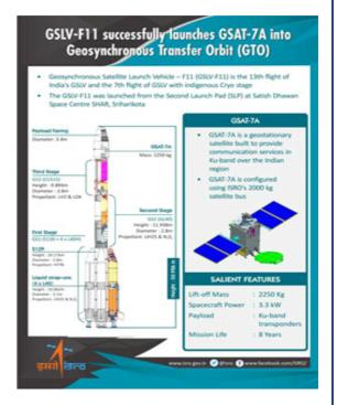
GSAT-7A is the 39th Indian communication satellite of ISRO to provide services to the users in Ku-band over the Indian region. Most of the functional requirements of the communication payloads and the other systems have been derived from ISRO's earlier geostationary INSAT/GSAT satellites.
